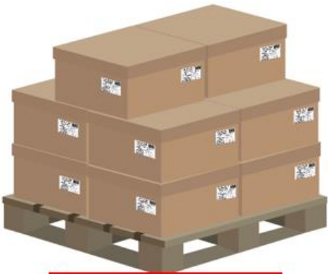
Incorrect; Must be complete layers
